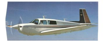
This is a four place single engine, low wing tricycle retractable gear aircraft with Lycoming 200 hp fuel injected engine and constant speed prop. It was used by myself for commuting in all weather conditions and maintained carefully in my personal hangar at Airlake (KLVN)in Lakeville, MN. It 's base color is 'sand beige'. It was built in Kerrville, TX and its manufacturer is still making later models. Many parts are still available.
